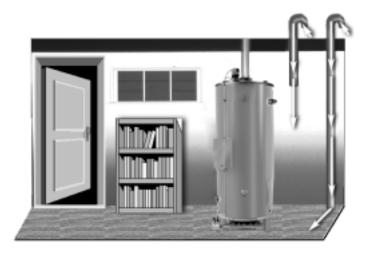
Again, two openings are required: one within 12 inches of the top of the enclosure and one within twelve inches of the bottom of the enclosure. Each opening must have a free area of not less than 1 square inch per 4,000 BTUH of the total input of all appliances within the enclosure.
